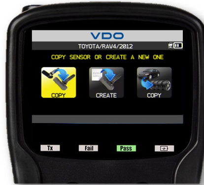
Copy and create TPMS sensor ID on all leading aftermarket programmable sensors
