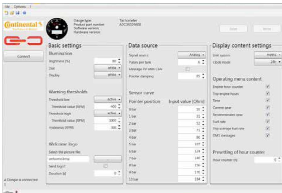
Exemplary illustration of the ConfigTool user mask. The set of items depend on the gauge variant
