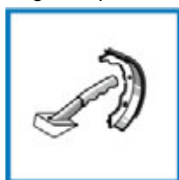
Drum brake shoes for parking brake
