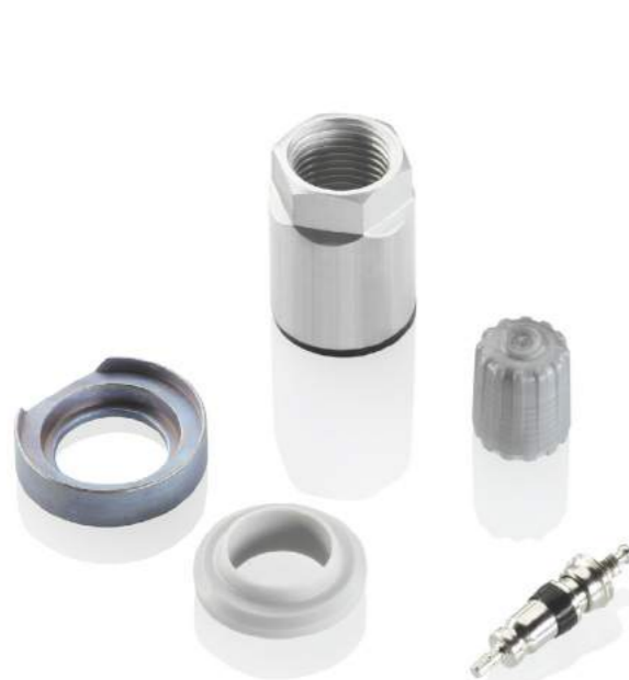
Service kit: valve insert, mounting nut, seal, seal washer and valve cap.
